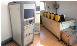
Test type: Angular contact ball bearing (7206)
