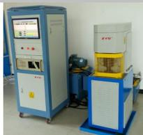
Test type: Ball bearing (steel / ceramic), thrust piece
